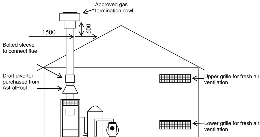
**An indoor draught diverter must be purchased from AstralPool and fitted to unit in accordance with AstralPool's Instructions and Installation Codes before the heater can be enclosed.**
