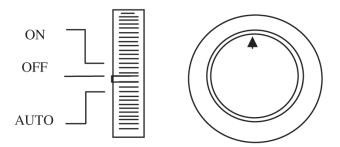
On - Over-rides automatic time clock, Filtration System switched on. Off- Over-rides automatic time clock, Filtration System switched off.
