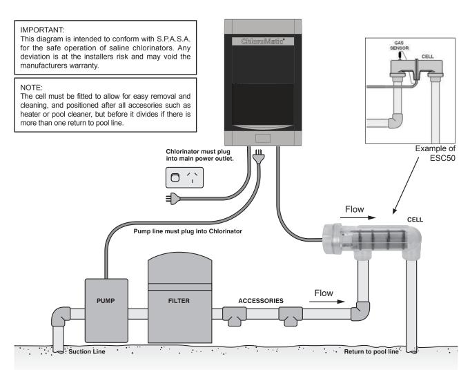
Two self-tapping screws and wall plugs have been provided for fast and simple installation. Simply cut out Template at bottom of page 19 for location of drill entry points. Use a 7mm masonry drill bit when fitting Power Supply to a brick or concrete wall. When mounting to a post drill pilot holes and fit screws provided. Once screws are in position simply hang chlorinator via bracket on back of Unit.
